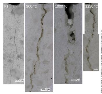
Figure 5. Example of research conducted at Forschungsgemeinschaft Feuerfest e. V. This image, which shows the crack path at different temperatures for fused silica bricks, is from a study on the fracture behavior of refractory materials up to service temperatures.
