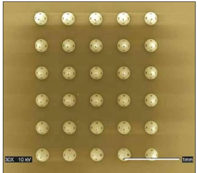
**Figure 6.** Ormocer microneedle array fabricated using 2PP. Arrays such as this can provide painless drug delivery and patient testing.
