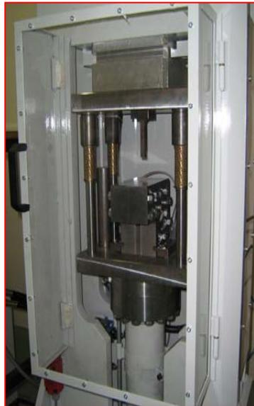
Equal-channel angular processing (ECAP)
