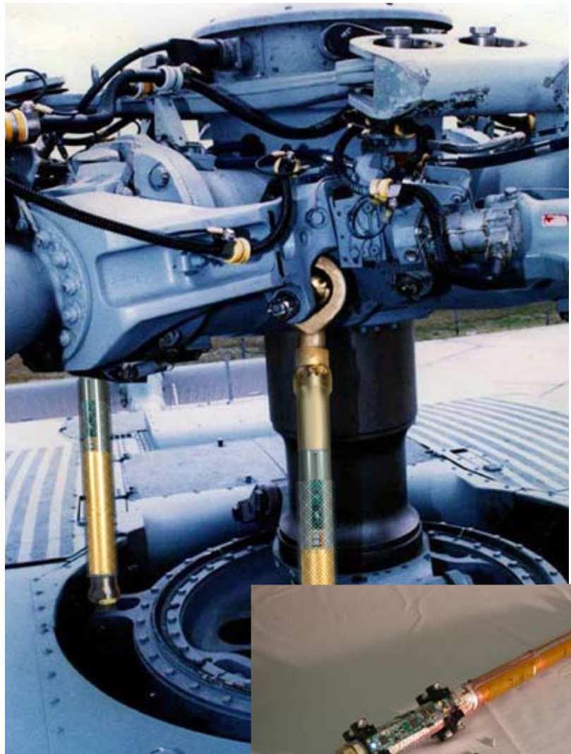
MicroStrain's harvester-sensor system takes its power from the cyclical strains of the same helicopter pitch link that it monitors for fatigue.
