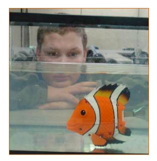
**IMPACT:** The fish could serve as an environmental data collection platform by adding communication, navigation, and environmental monitoring sensors.
