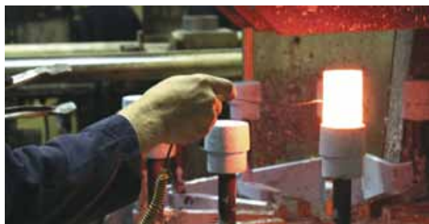
Some of Garrett's work is at VForge Inc. in Denver, Colo., where induction heating is used to reheat the 55vol% TiC/45vol% Al composite cylinders to 1150°C for the die casting process.
