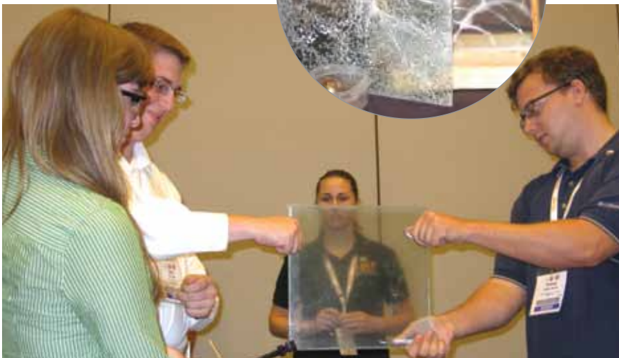
Fig. 2 These students are participating in one of the demonstrations that will be included in the kit. The students are learning the strength of safety glass, which is thermally tempered, compared with the strength of glass that hasn't been tempered.
