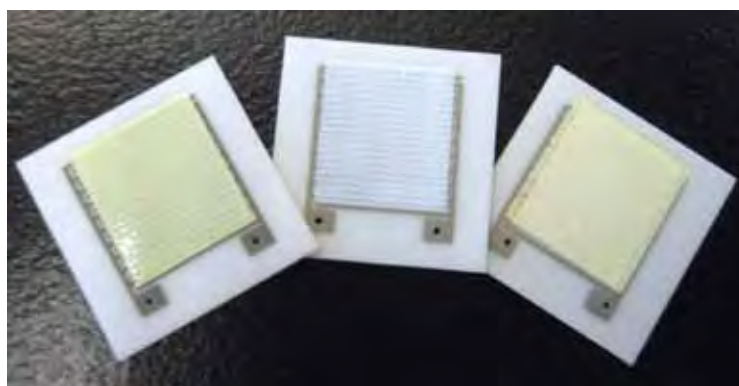
Metal-oxides printed on alumina sensor substrates with integrated platinum electrodes. Left to right: \text{WO}_3 , \text{SnO}_2 , and Nb-doped \text{TiO}_2 .
