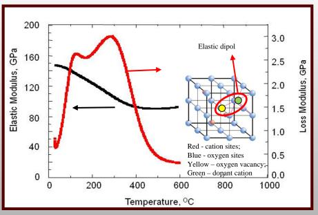
Elastic and loss moduli of 8mol%  $Y_2O_3$  stabilized  $ZrO_2$  determined by DMA.
