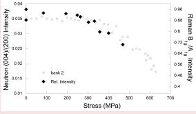
Using Raman spectroscopy to measure the coercive stress and process zone size of ferroelastic ceramics we can understand the relationship between toughness and doping regimes
