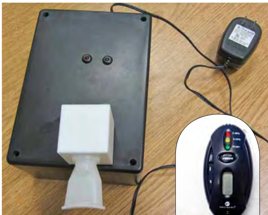
**Figure 3** Prototype of an acetone breathalyzer for monitoring diabetes and diet control. The circuitry of the “black box” is shown in Figure 1. Inset: A keyring version of a commercial alcohol breathalyzer shows the potential for affordable, portable diagnostics tools.
