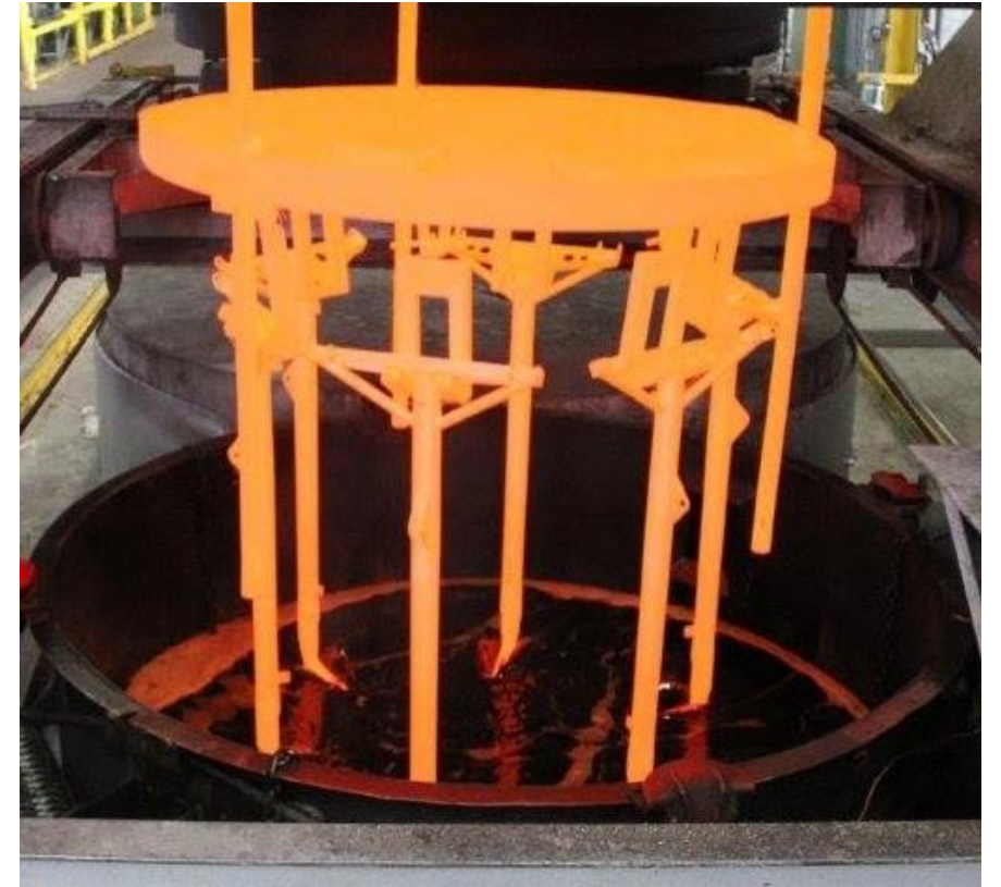
Aircraft landing gear glowing red-hot, about to be quenched in oil
