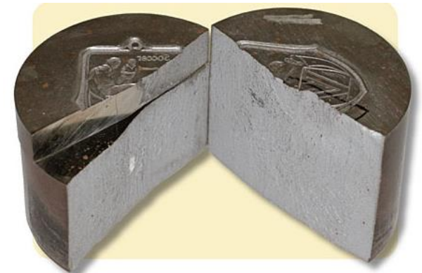
Steel quench crack
