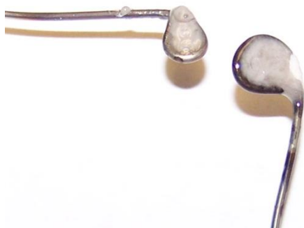
Figure 6. Beads that have a gray, milky color rather than a transparent, bright color due to the gas bubbles that remain trapped in the amorphous Borax
