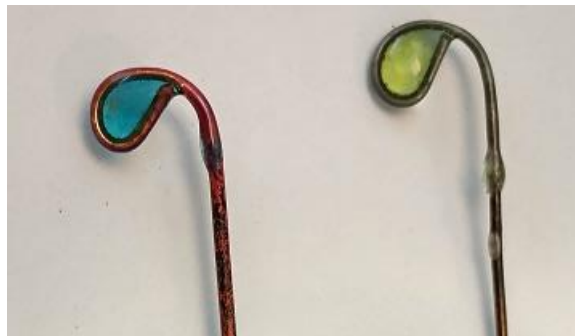
Figure 4. Borax beads formed with copper wire (blue bead) and nichrome wire (green bead)
