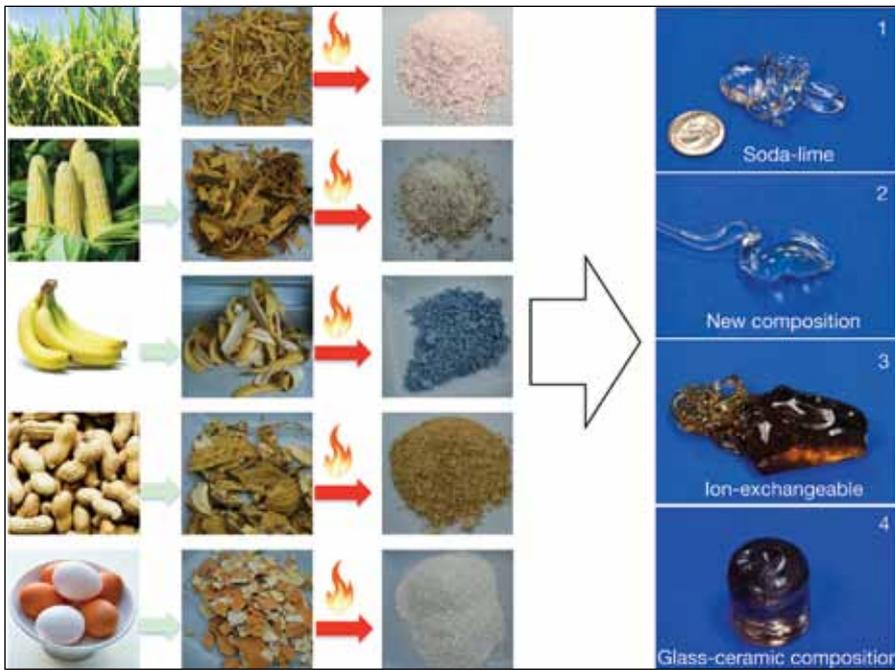
**Figure 2.** Raw materials are produced by grinding and heating food wastes. Four glasses made from these wastes are shown at the right with a U.S. dime shown for scale.
