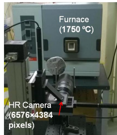
Fig. 8. High-temperature furnace with a high-resolution camera.
