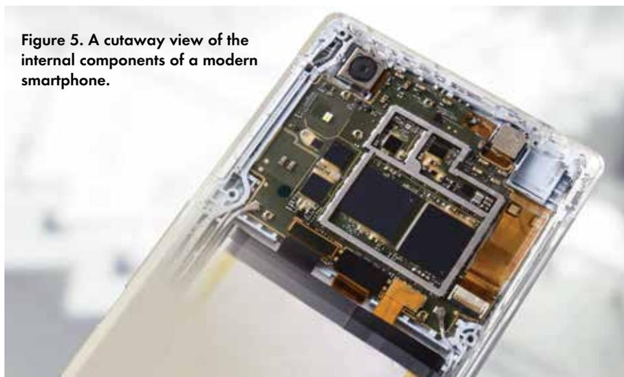
**Figure 5. A cutaway view of the internal components of a modern smartphone.**
