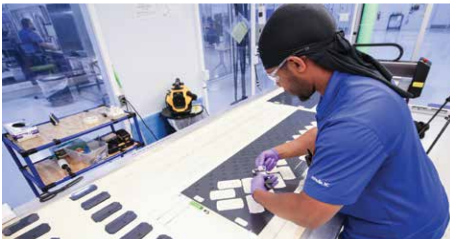
Figure 4. Ply shapes being removed from a tape immediately after ply cutting operation has been completed. Asheville, N.C.
