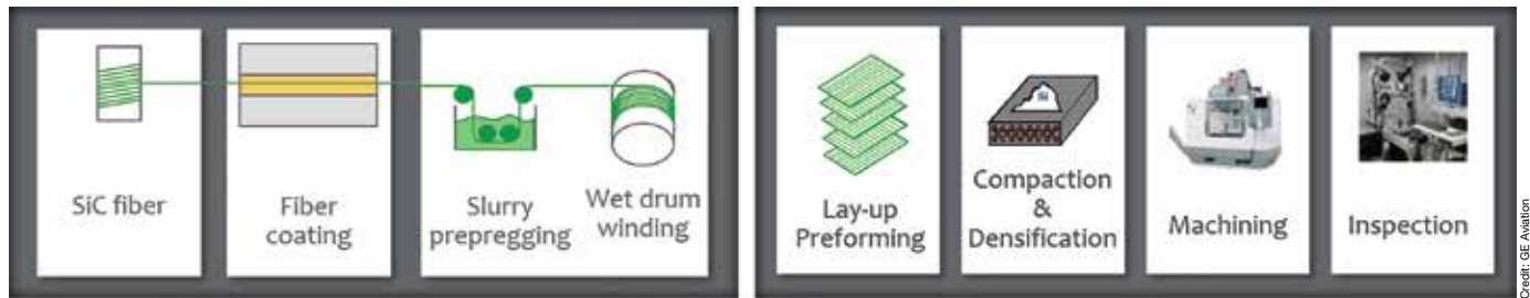
Figure 3. Prepreg/melt infiltration process flowchart for fabricating SiC/SiC CMC components. The final step after component fabrication is to apply an environmental barrier coating.
