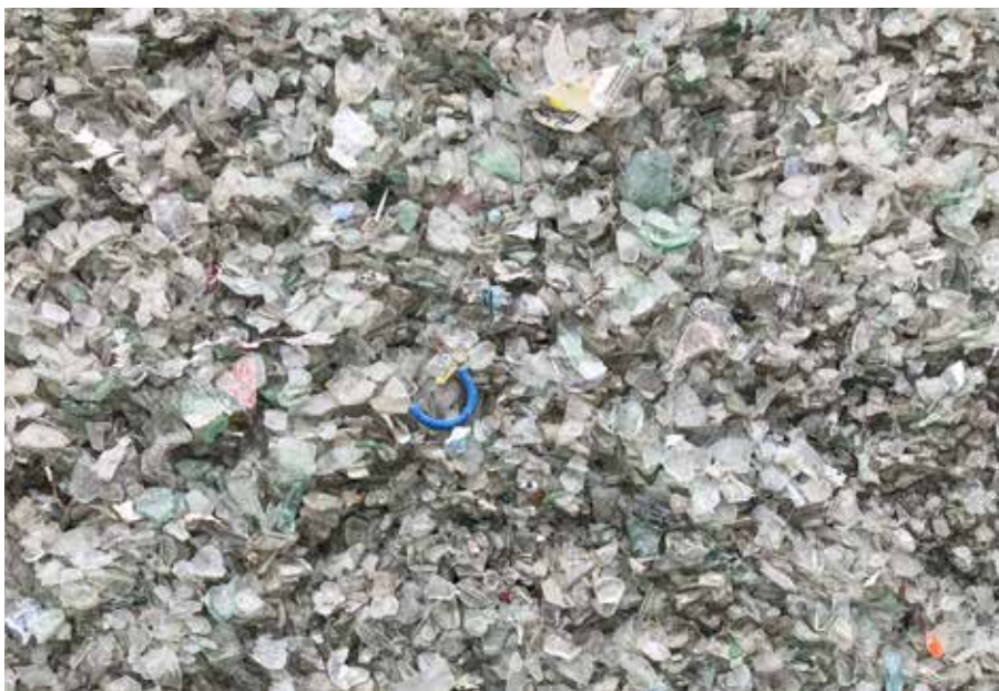
Figure 2. Example of post-consumer cullet that has been color-sorted into flint and is ready for reuse in a glass container furnace.
