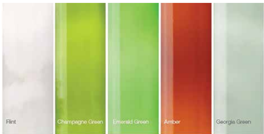
Figure 3. A selection of typical commercial glass colors. Many additional colors are also possible and controlled by composition and redox.
