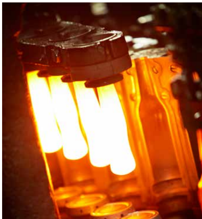
Figure 5. Parisons entering the final blow mold of a forming machine. This is a quad machine, meaning that four bottles (from four gobs) are simultaneously made in one section of the machine.
