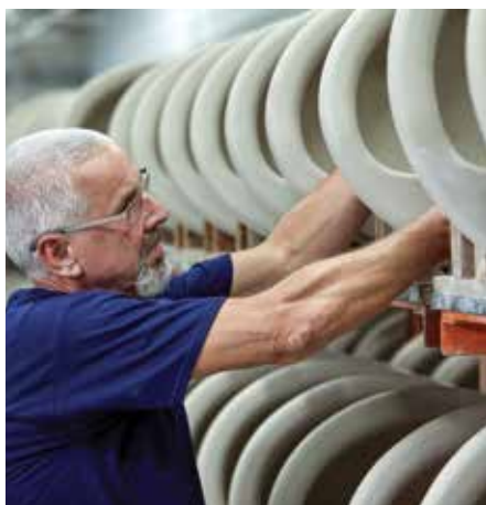
Figure 6. A worker at Mansfield Plumbing loads a batch of slip cast washbasins on the transportation cart. Ceramic engineer manager Felipe Mejia says the sanitaryware industry is looking to automate the more labor-intensive steps of the manufacturing process.
