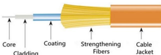
**Fiber Optic Cable Construction**
