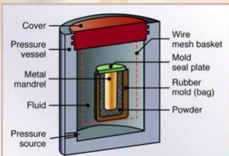
Cold isostatic pressing allows the fluid to uniformly compact the particles into a sphere.
