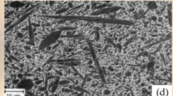
(a) Silicon nitride is often made into ball bearings to assist in rotation and reduce friction in rotating machinery. (b) The ball bearings are can be implemented in axle systems. (c) The material can be made into a variety of useful shapes for high-temperature applications. (d) We are able to see how the needle-like grains are arranged on a fine scale by using advanced microscopes.
