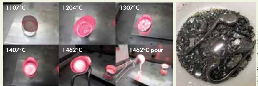
(left) Melt series based on chemistry of melted amphibolite composition from the Broborg site. Melting in atmosphere and without the use of bellows required heating the material to temperatures >1,400°C, which is not likely to be reached in ancient times. (right) Final glass produced from the melting study.
