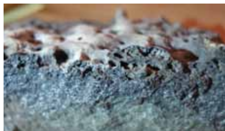
Figure 2. Examples of hillfort glasses, which are manufactured glasses with compositions similar to some nuclear waste glasses. An amphibolite rock source for vitreous material, found at Broborg in Sweden, shows a molten top portion.
