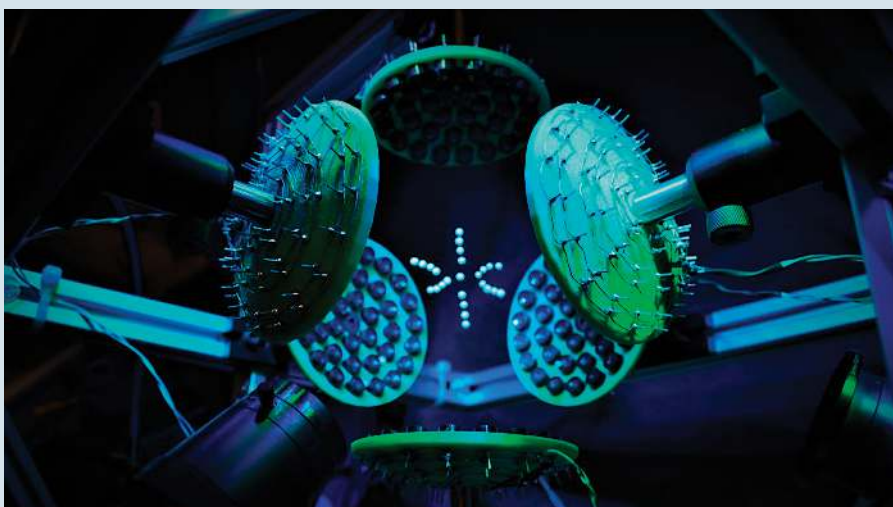
A three-dimensional sound field created by Materials Development Inc. enables levitation of 25 styro-foam spheres. The process allows for measurements using neutron methods to study how liquids change into glass and to investigate extreme temperature processes. Credit: Materials Development Inc.
