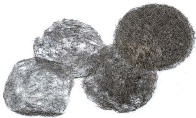
Figure 7. Nonwoven veils produced from LP30-SC short SiC fibers.
