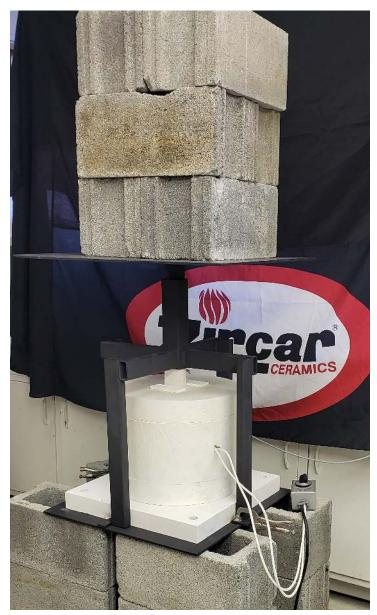
Pictured above is ZIRCAR Ceramics' Creep Testing Apparatus wherein a 250psi load is applied to a 1" cube sample. Data was collected after one hour at 710°C, 810°C, 910°C, 1010°C, and 1110°C.
