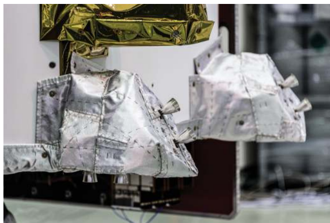
Figure 6. Close-up of a set of thrusters on the BepiColombo Mercury Transfer Module that will carry the two science orbiters—the Mercury Planetary Orbiter and the Mercury Magnetospheric Orbiter—to the innermost planet. The silver/white thermal blanket is covered with Nextel, a ceramic cloth known for its heat-resistive properties, which will allow the thrusters to be exposed directly to the sun.
