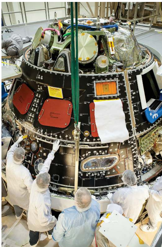
Figure 4. Inside the Operations and Checkout Building high bay at NASA's Kennedy Space Center, technicians dressed in cleanroom suits have installed a back shell tile panel onto the Orion crew module and now are checking the fit next to the middle back shell tile panel.
