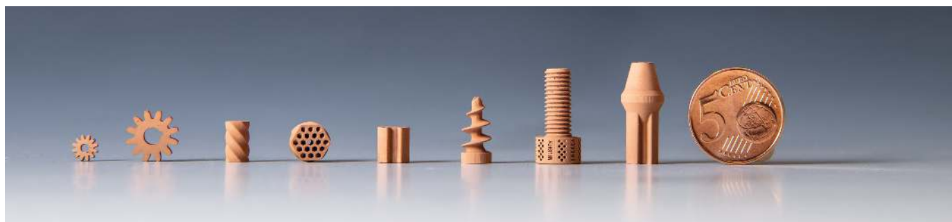
Figure 11. Finely detailed ceramic parts that were 3D printed using simulated lunar regolith. The European Space Agency and Lithoz collaborated to investigate how 3D printing could be used to support a lunar base.
