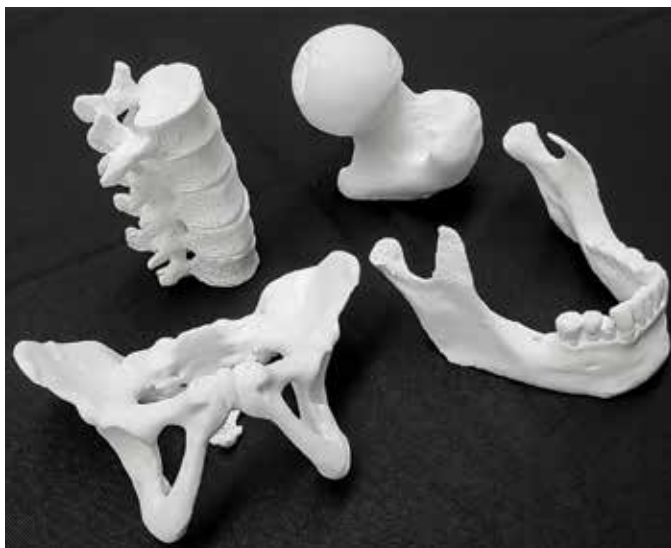
Figure 9. Anatomical structures display a handful of possible structures that were 3D printed by Dimension Inx with Hyperelastic Bone: (clockwise, from top left) spine, femoral head, mandible, and pelvis.
