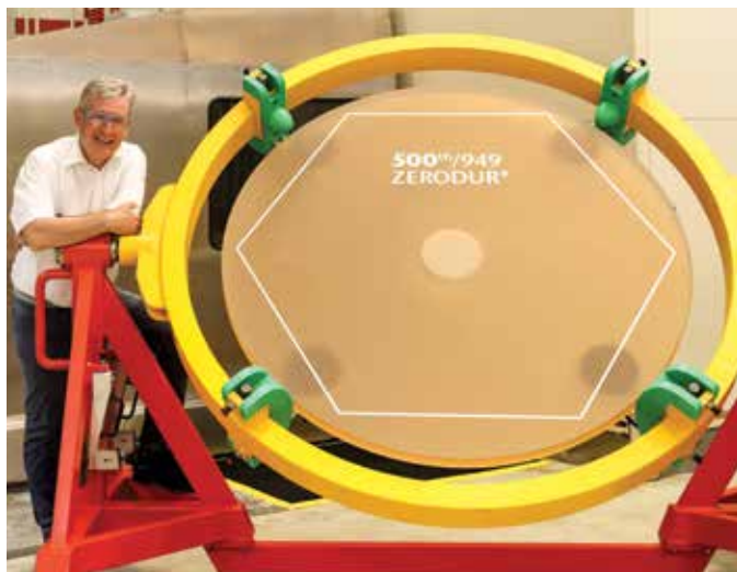
Figure 3. Thomas Werner, head of the Extremely Large Telescope project, pictured with the 500 th ZERODUR mirror blank for the M1 primary mirror.
