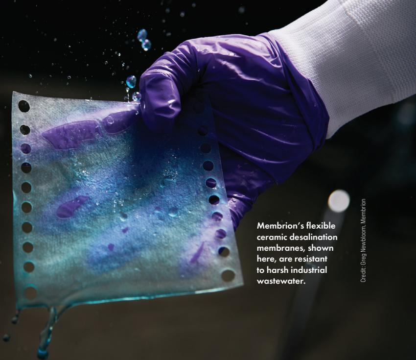
Membrion's flexible ceramic desalination membranes, shown here, are resistant to harsh industrial wastewater.
