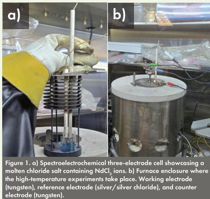
Figure 1. a) Spectroelectrochemical three-electrode cell showing a molten chloride salt containing  $\text{NdCl}_3$  ions. b) Furnace enclosure where the high-temperature experiments take place. Working electrode (tungsten), reference electrode (silver/silver chloride), and counter electrode (tungsten).
