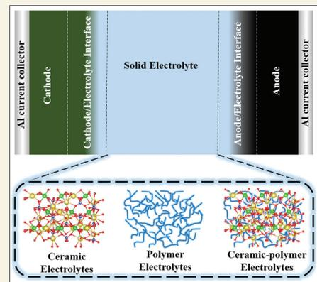
**Figure 1. Schematic demonstration of a typical all-solid-state sodium battery comprising an anode and cathode integrated with various categories of solid electrolytes.**
