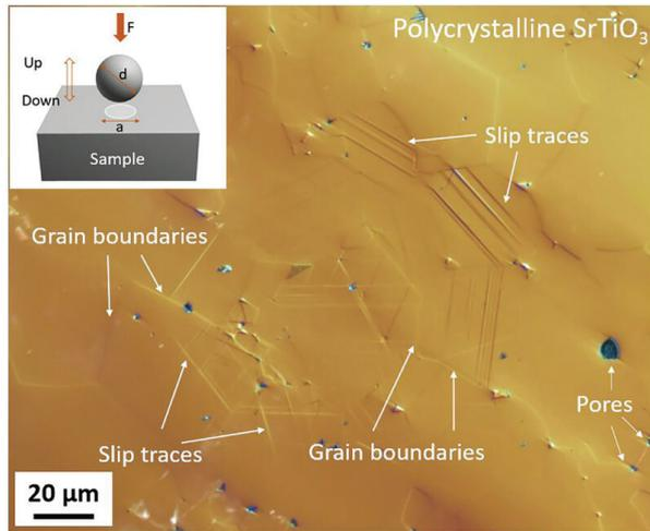
**Optical microscope image highlighting the slip traces induced by Brinell indentation (inset) on a polycrystalline strontium titanate sample at room temperature.**
