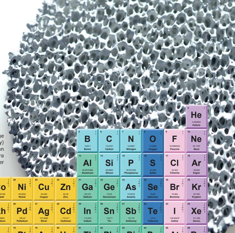
Photo: Ceramic sponge (nanoscale morphology) produced from American Elements proprietary ultra high surface area powder
