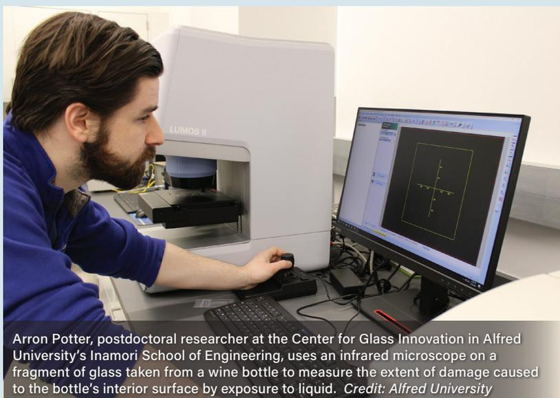
Arron Potter, postdoctoral researcher at the Center for Glass Innovation in Alfred University's Inamori School of Engineering, uses an infrared microscope on a fragment of glass taken from a wine bottle to measure the extent of damage caused to the bottle's interior surface by exposure to liquid. Credit: Alfred University
