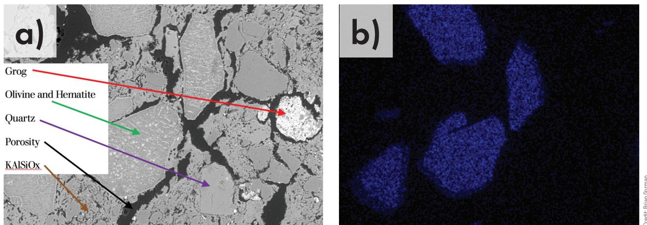
**Figure 1. a) Backscattered scanning electron micrograph of the clay brick sintered microstructure. b) Energy dispersive X-ray microanalysis spectral image of the same area illustrating the location of magnesium. Magnesium is retained within the olivine grains, which are well dispersed within the microstructure. Abundant pore-olivine interfaces are also observed. Horizontal field width = 600 mm.**
