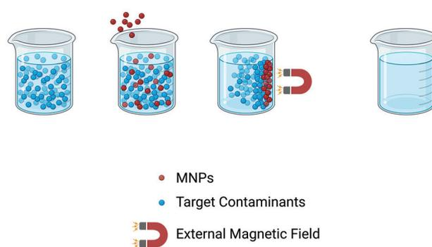
**Figure 1. Schematic demonstrating magnetic separation. Contaminating blue particles are sorbed by magnetic red particles and then separated out using an applied magnetic field.**
