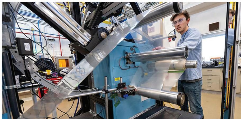
The National Renewable Energy Laboratory's roll-to-roll web line is used for research of in-line quality control monitoring techniques for battery, electrolyzer, and fuel cell materials.
