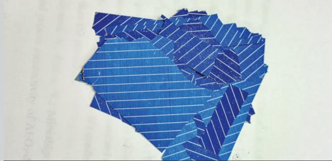
Example of clean pieces of silicon extracted from discarded solar panels using thermal delamination.
