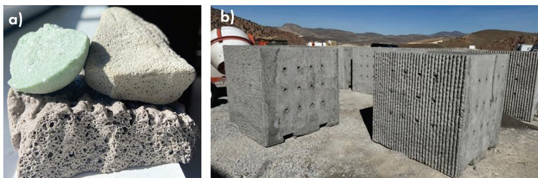
**Figure 3. a)** Images of varying foam glass compositions. The green foam glass (left) is SilicaX's aggregate, while the traditional grey foam glass (top) and experimental foam glass (bottom) were created by Collin Wilkinson's group at Alfred University. **b)** SilicaX coupons being produced for immersion in the Long Island Sound.
